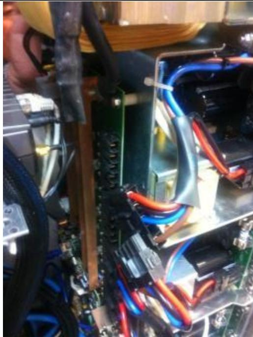
Once all the screws have been removed, a screw is used to separate the unit from its support
